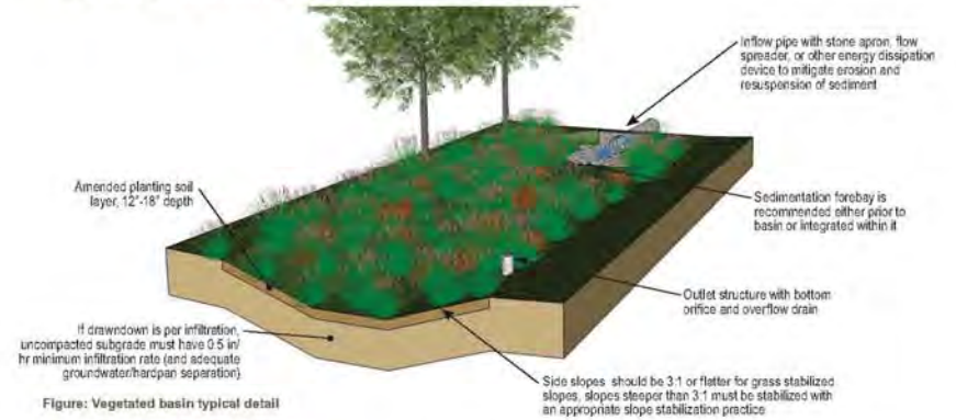
Figure: Vegetated basin typical detail
