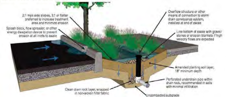
Figure: Vegetated swale typical detail
